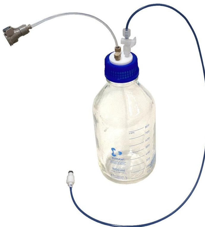
Fig. 1. ET 210 glass bottle assembly for use with the acidic mobile phases for separation.
